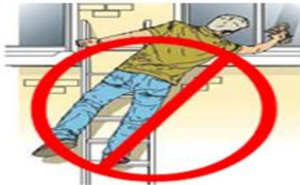
Figure 4 Over Reaching the Ladder's Center Position
